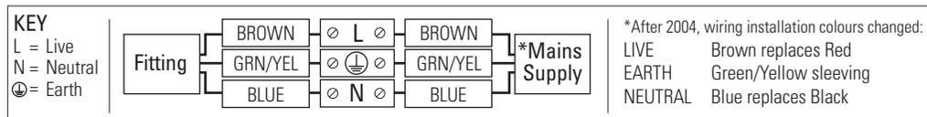
9. Double check all the connections are secure and that no loose strands of wire are left out of the connector, ensure that the lid of the terminal block is closed securely after making the connections.
